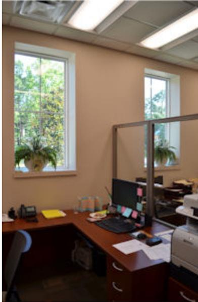
Fundamental building commissioning, daylight and occupancy sensors, and interior lighting power density less than 0.8 watts per square foot, all contributed to the building energy performance being 30-35% above minimum Florida Building Code requirements.
